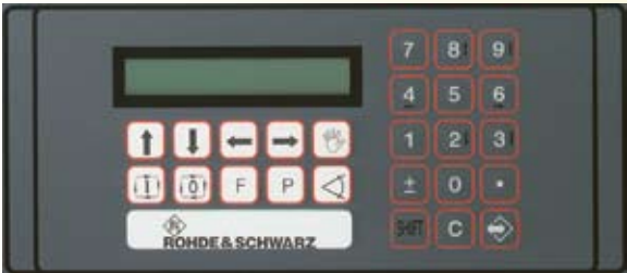
Control section and LCD display of the R&S®GB 130
