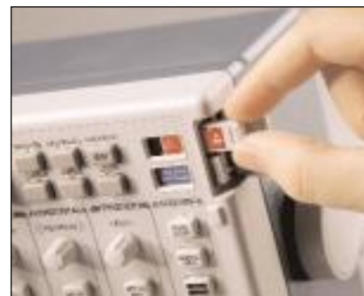
Application Module being installed.
