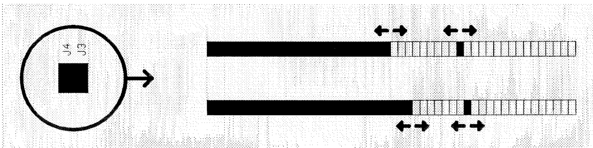
Afb 4: LED-bar with slowly dropping peak-hold-dot
